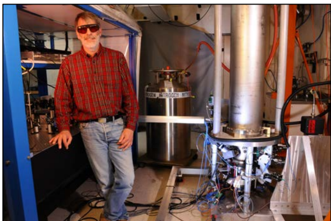
NIST-F2 laser-cooled fountain standard atomic clock
